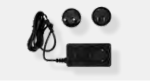
Alimentatore a spina con connettore 3.5/1.3 (Pencil modulo luce, Pencil base ricarica) Charger with a 3.5/1.3 connector (Pencil lighting module, Pencil charging base) 48W INPUT: AC 100-240V | 50-60Hz OUTPUT: 19 V - max 2,5 A LD0800CS
